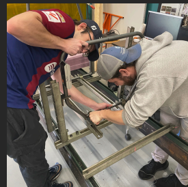
JIGGED UP THE CHASSIS FOR WELDING
