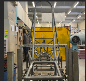
FINISHED WELDED CHASSIS
